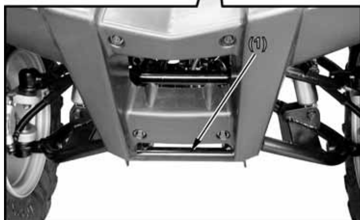
(1) Location of Frame Serial Number
