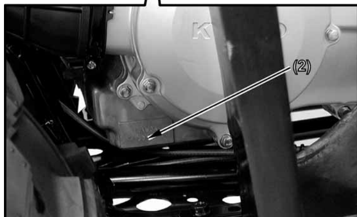
(2) Location of Engine Serial Number
